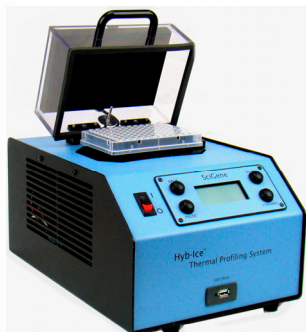
Hyb-Ice unit with 0.2ml PCR block.
