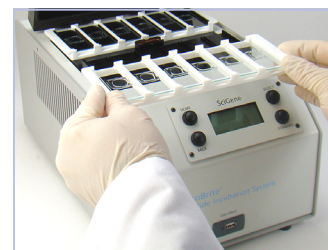
After denaturation on the CytoBrite System trays are moved to the oven.
