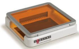
The UltraSlim blue LED transilluminator is ideal for safely imaging gels stained with SYBR Safe, Gold and Green, GelGreen and UltraSafe blue.
