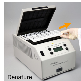
Fig 5. Denature at 76° for 2 min.
