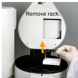
Fig 10. Take rack from centrifuge.
