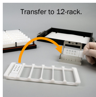
Fig 8. Transfer slides to 12-rack.
