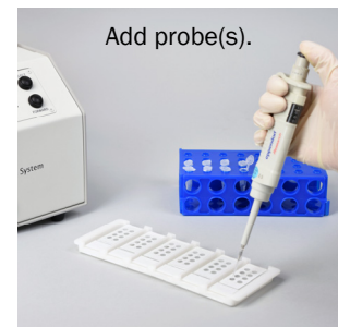
Fig 3. Pipette 1µl probe into wells.
