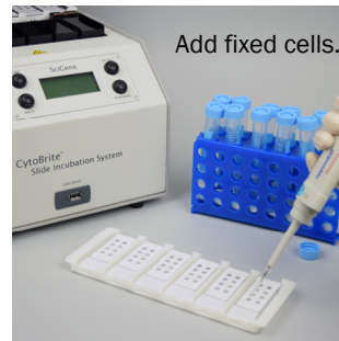
Fig 1. Pipette 1µl fixed cells into wells.
