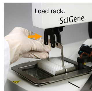
Fig. 9. Load rack onto gripper.
