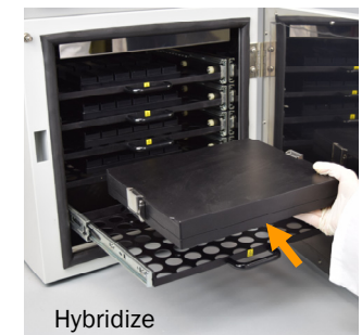
Fig 6. Transfer CytoBrite slide trays to hyb chamber and place in oven.
