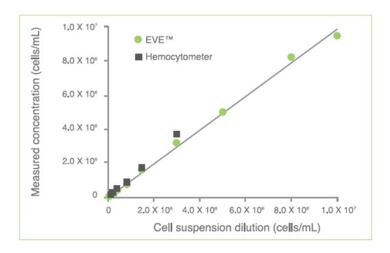
Measuring from the EVE™ extend further along the high concentration range than hemocytometer readings.
